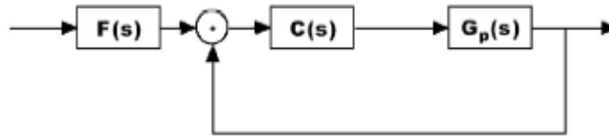
Figure 4.5 QFT Feedback Structure used for the Fractal Controller {28}
